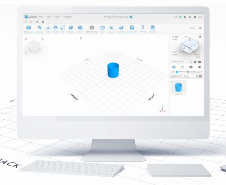
**Add Thickness** allows you to add volume to your models, and its basic usage is to add thickness to open figures (such as containers) to print them with a more sturdy frame.
