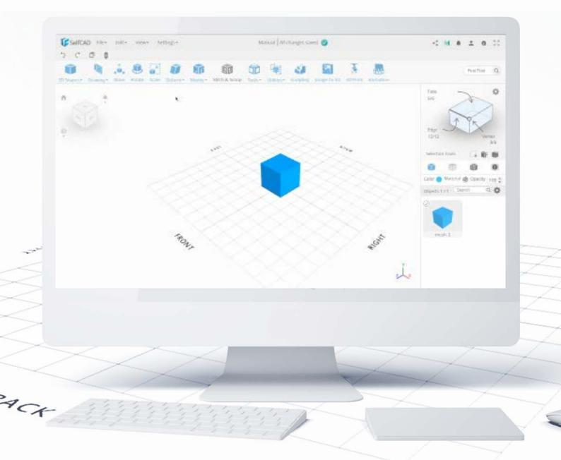
You should know by now, that tools in SelfCAD have very obvious names. **Skew** allows you to simply skew the figure, and just like it's been the case with <u>Transformation</u>, you can do it either by dragging respective gizmos in a certain direction or by typing in the numbers.
