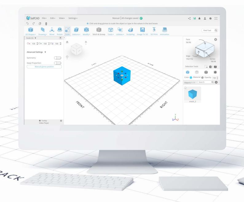
**Scale** works in the exact same way the previous two tools did, but you'll find here 2 additional options - one to keep the **Symmetry** and the other to **Keep Proportion**. **Symmetry** scales the object in both directions on a single axis, and **Keep Proportion** scales in equally in all dimensions.
