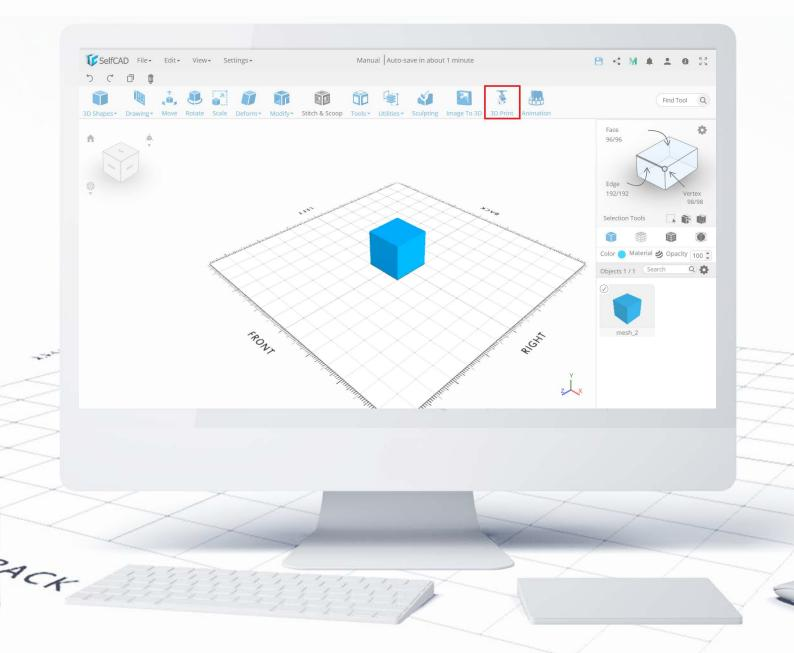
Almost at the end, you'll find the option to **3D Print** your design. This tool will slice the object, and generate a GCode in preparation for 3D printing. It might sound complicated, but you don't have to worry - all of that is being done automatically by the software for you.
