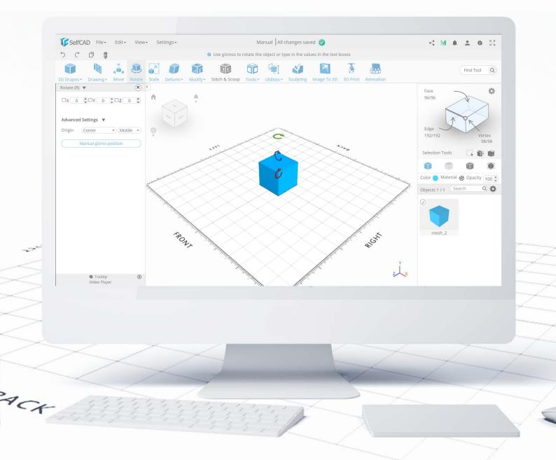
The **Rotate tool** works on the same principles as the <u>Move tool</u> - you can drag the gizmos on the screen to rotate your object or type in the exact angle you want to rotate it.
