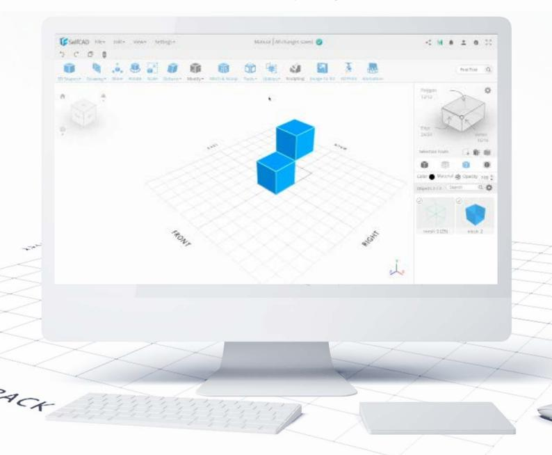
**Merge Objects** allows you to connect objects without changing their geometry. It works correctly when the shapes you want to merge do not overlap each other otherwise it will create an unwanted problems during printing.
