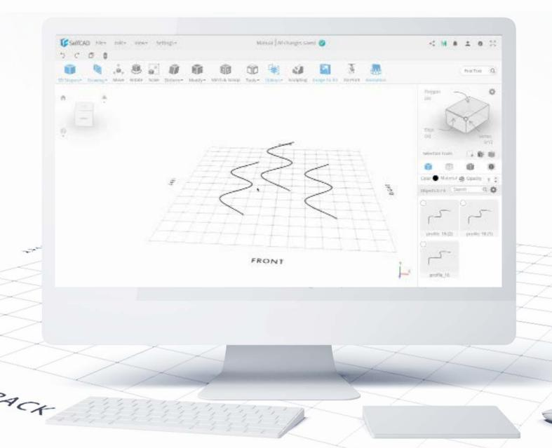
The **Loft** tool creates connections between shapes and profiles - it connects their outlines to create a solid shape. Previously, I said that Sketches serve as a foundation, then you can think that Loft pours the concrete over the foundations. There are a few options to slightly customize the Loft with Fill and Bevel Settings, with which - at this point - you should already be familiar with.
