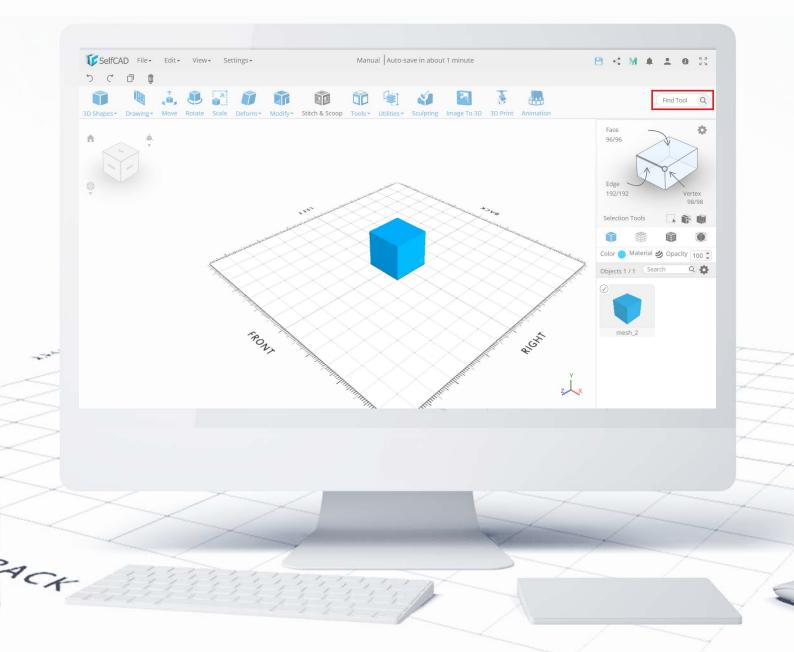
At the end of the panel, you'll find a **Search Tool** feature - with it, you can simply type in the name of the tool to get quick access to it. Also, because the tools in SelfCAD have names that reflect their function, you can simply type in what you want to do with an object, and the software will provide you the tool for that purpose.
