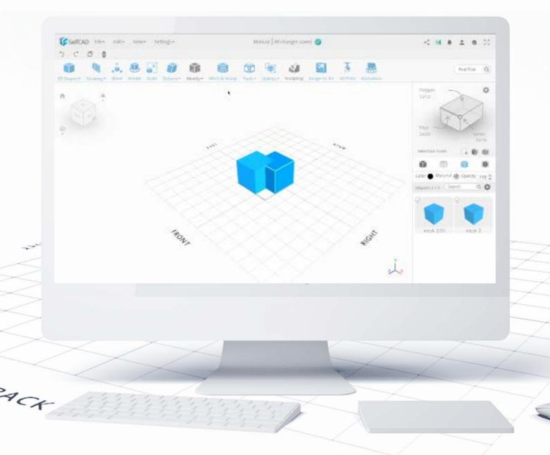
**Union** connects two (or more) objects into one and completely changes the geometry of the now united figure. It makes sure, that there are no edges left from previous figures hidden inside the new model, that could later interfere during printing.
