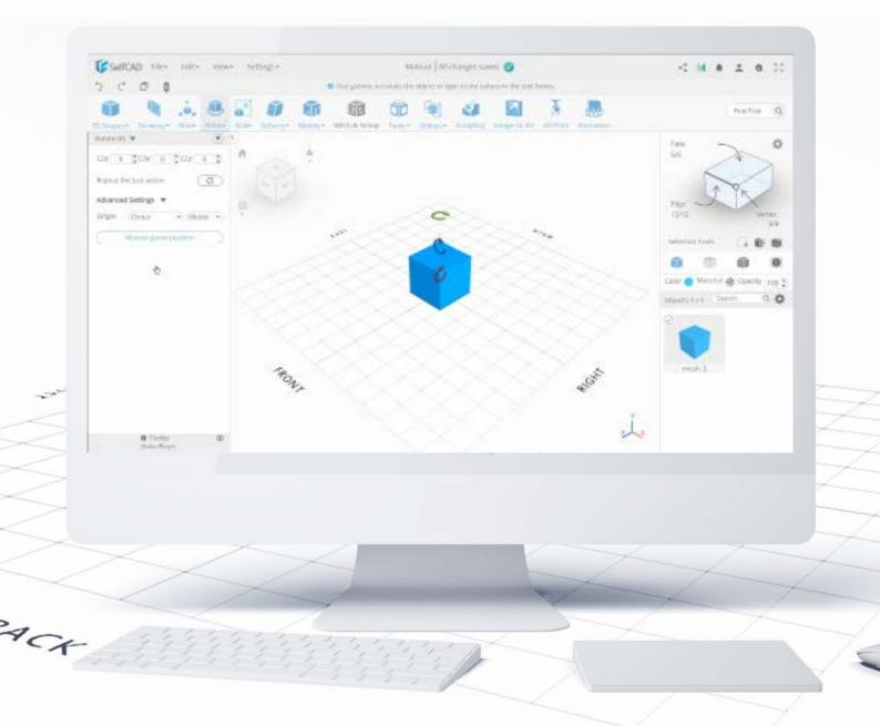
One of those advanced settings is the **Gizmo's position**. You can think about it as a point of reference - it sets up the origin around which the tool will apply the change. For example, the Gizmo's position in the Rotate tool allows you to choose around which Edge the figure will be rotated.
