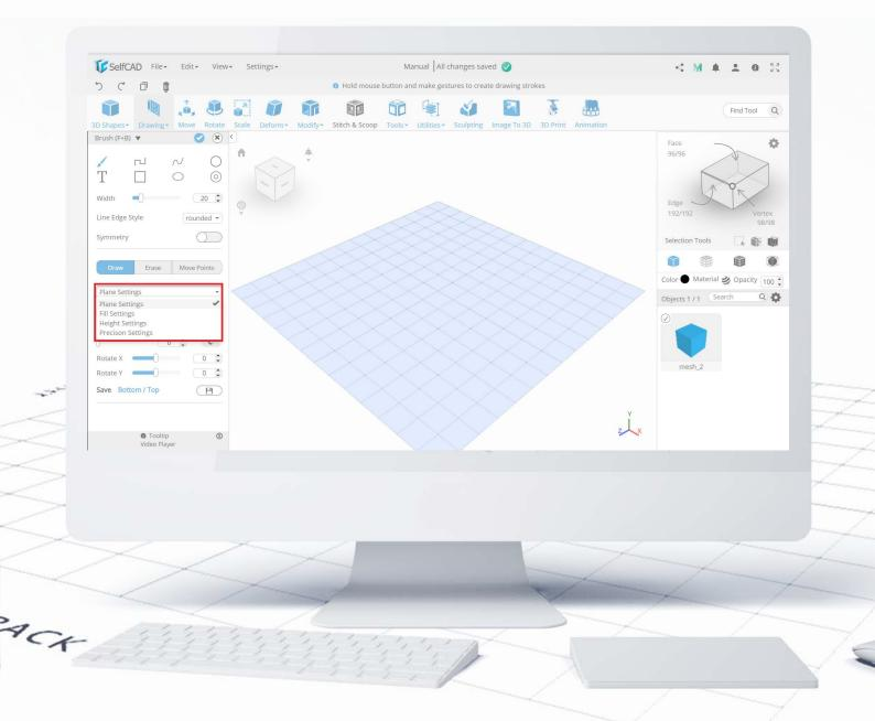
In the end, you'll find options to customize the already drawn object: **Plane Settings** allow you to specify the **Offset (position)** of the drawing, **Fill Settings** allows you to choose between creating **Solids** and open figures, **Height Settings** changes the thickness of the 3D model, and **Precision Settings** can be used to snap your drawing to other Shapes, **Guides or Grid Vertices**. You can also set the **minimum length and angle** of each step.
