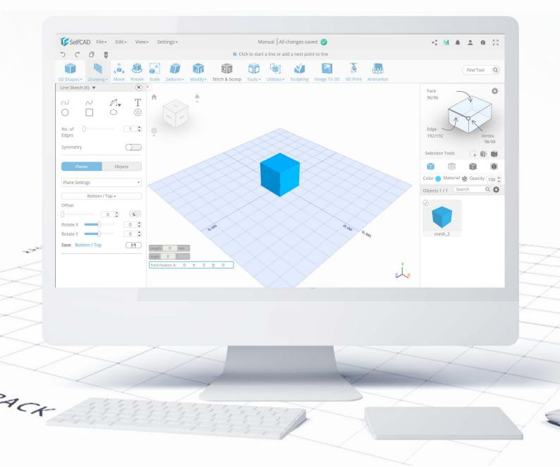
**3D Sketch**, on the other hand, works differently - it serves as a tool that builds a frame that you can later fill up with the help of other tools. It's like setting up a foundation upon which you'll create the complete model with the help of other tools.
