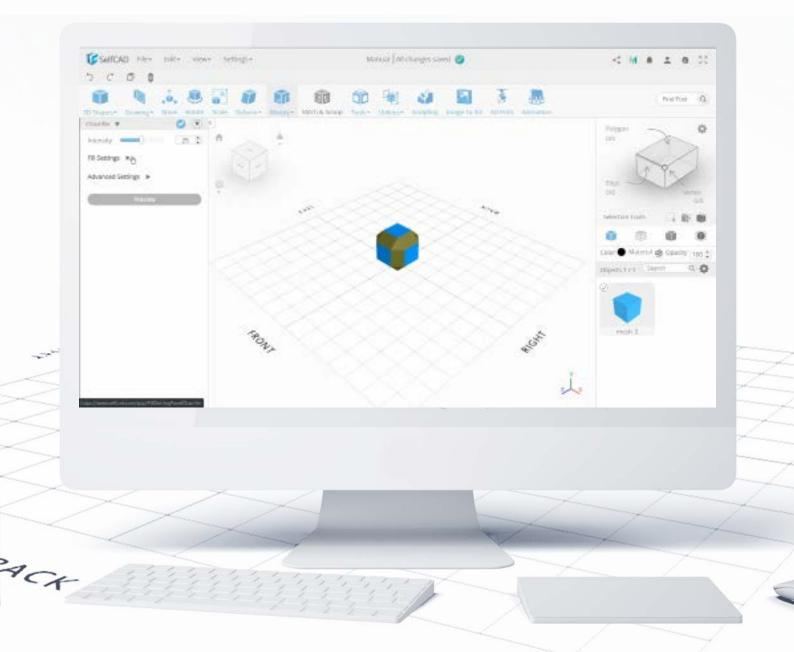
As I said, the **Fill Settings** allow you to choose which parts of the figure you'd like to keep after beveling, and you can choose from Polygons, Edges, and Corners. In the advanced settings, you can set the intensity of the bevel to be based on length or percentage.
