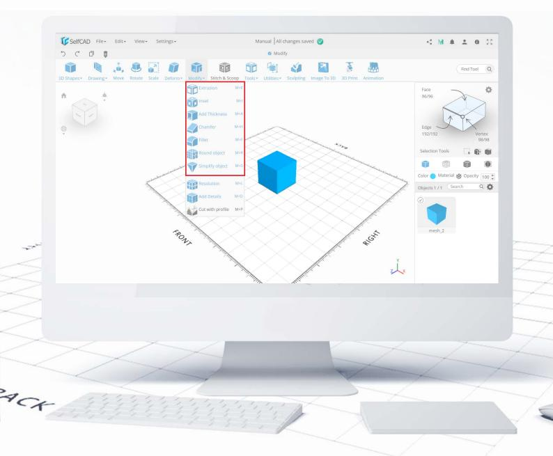
The tools above the divider will change the way how your objects look, as well as how they are constructed - each time you use one of these tools you'll alter the geometrical shape of your figure by basically cutting out a piece of the 3D model.
