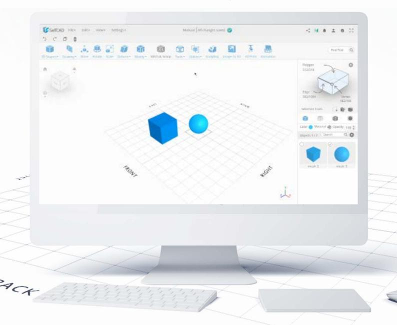
As its name suggests, you can use this tool to align one object to another. There are options to choose to what exactly do you want to align your figure - you can align 3D models to other figures in the grid, or the grid itself, select which part of the figure should be aligned and even set precise offset (distance) between the aligned objects.
