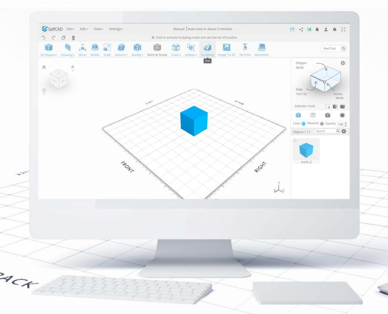
Next in line is **Sculpting** - out of all of the tools available for modeling, this one can be the most precise of them. You can use it to add the most minute details and finishing touches to your designs. Sculpting works in a completely different way from other tools - here you don't manipulate the object directly by changing the settings of the tool, but by using different brushes directly onto the object itself to invoke a change.
