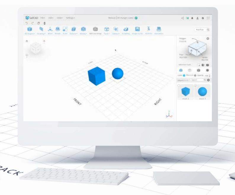
**Snap** allows you to immediately move selected shape to any place on the grid or onto any model. There is also an option to set the offset between the model and the point you want to snap it to.
