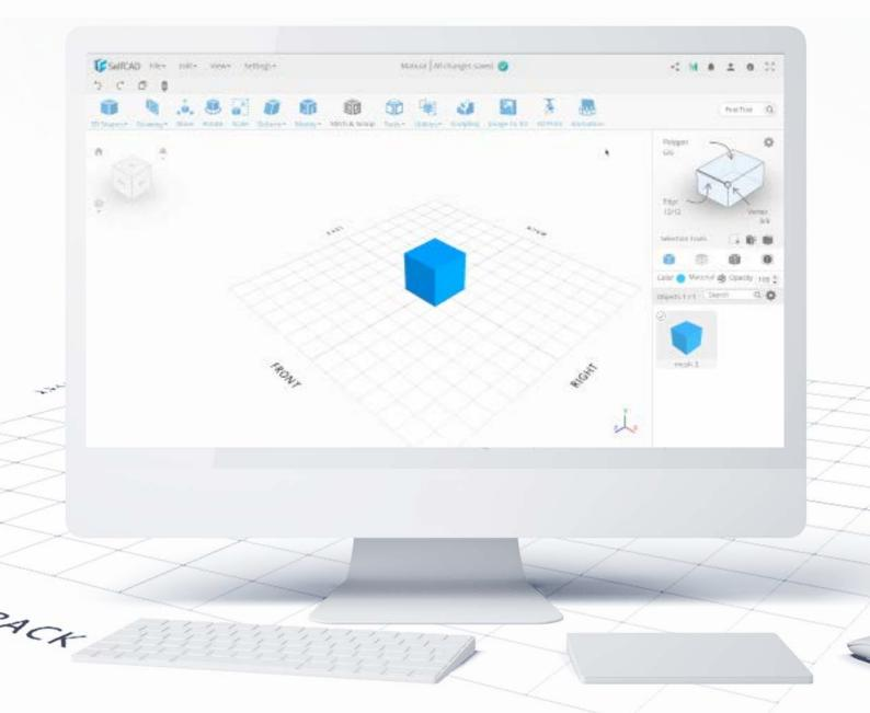
And the latest addition to the software - the **Animation** tool. In short, it allows you to record everything you do in the software. Each action becomes a separate slider on the timeline, so you can later overlap and stack them together, to make it look like multiple changes were added to a model at the same time. When all is set, you can download the animation in the GIF format.
