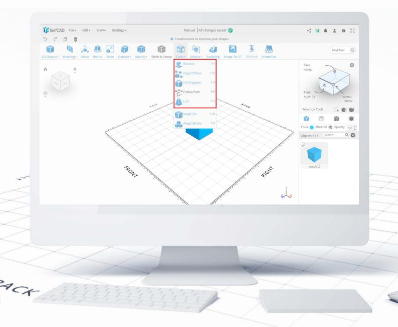
Tools above the divider are dedicated to working on, and improving primitives, drawings, and sketches, and turning them into more complex 3D models. They focus mostly on connecting profiles, filling empty spaces in polygons and arranging them in specific patterns.
