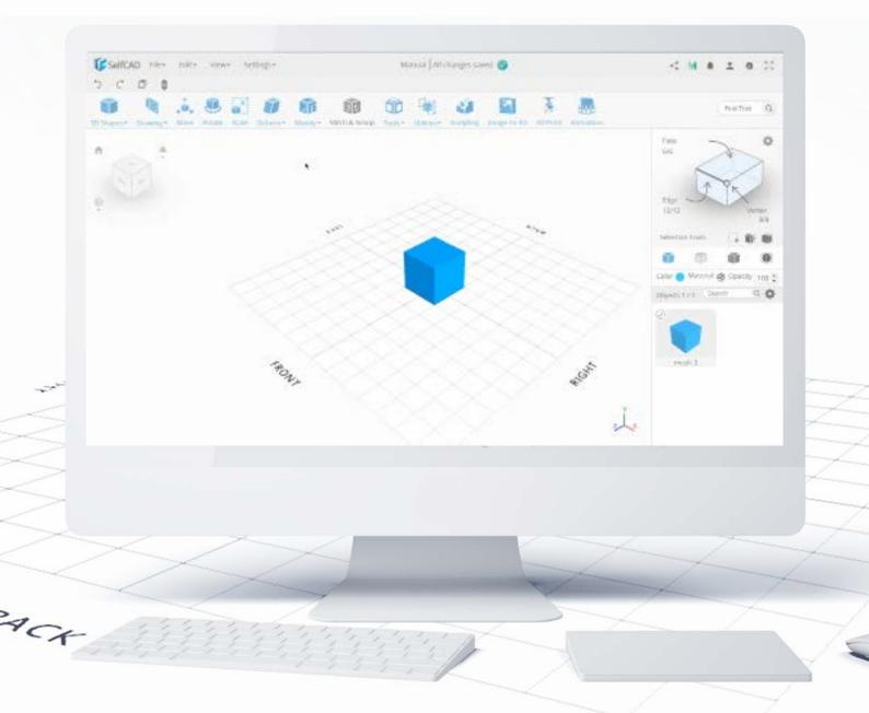
**Extrusion** in its default form allows you to extrude polygons of the figure, and you can manipulate the value of the extrusion by operating a slider - the positive value will extrude the polygons outwards, and the negative value will extrude them inwards.
