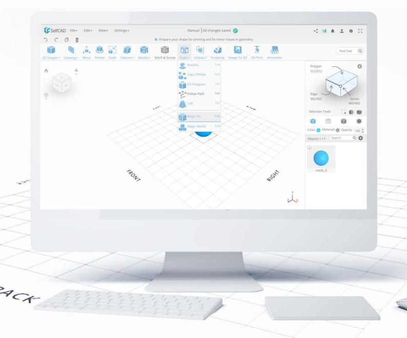
**Magic Fix** is a tool that rebuilds your objects by removing small, unprintable details. It's a good practice to use this tool before printing - this way you'll always be sure that there are no problems with the geometry of your project.
