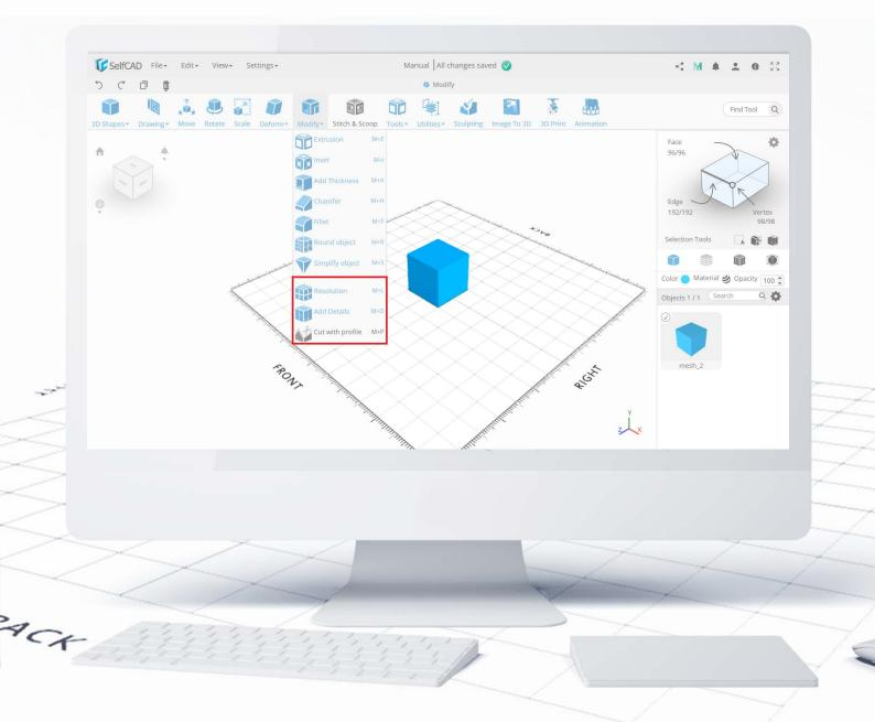
The tools below the divider don't change the shape of the model, but they change the shape and the number of segments that the figure consists of.
