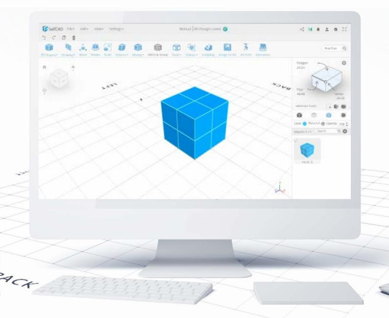
Add Details allows you to manually increase the level of detail of the figure, by splitting existing faces into smaller ones. You can do it either by clicking on the figure to add Vertices or by dragging an existing edge to its neighboring face to create a new edge there. The automatic loop finding will do its best to add edges all around the model.
